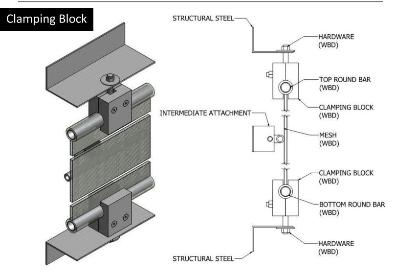
Attachment Specifications MAX MESH HEIGHT: 20' | MAX MESH WIDTH 20' | TYPICAL INTERMEDIATE SPACING: 10'
